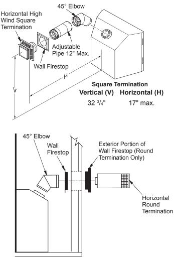
Figure 14 - Horizontal Termination Configuration for Square or Round Termination
